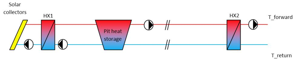
**Figure 3.5. Principle diagram of a simplified solar loop model, where all solar heat produced goes to the PTES.**
