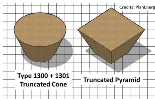
**Figure 3.2. Heat storage geometry used by the TESS component “Type 1300+1301” compared with actual geometry of the PTES in Dronninglund.**
