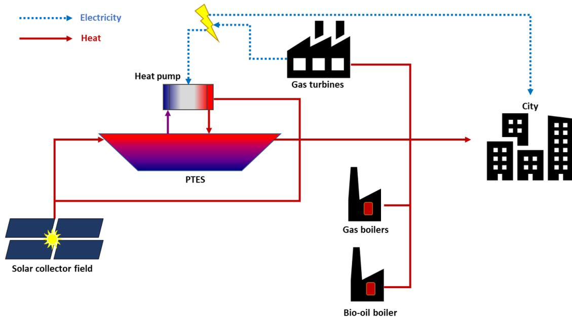
**Figure 3.7. Schematic showing the main elements of the system model for Dronninglund and which elements they can deliver heat (and electricity) to.**
