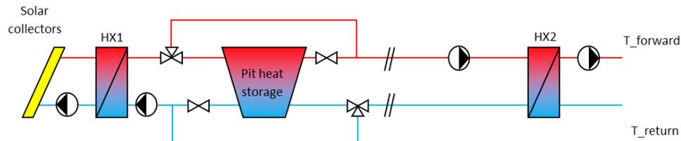
**Figure 3.6. Principle diagram of a more detailed solar loop model, with an option to send solar heat directly to the district heating network.**
