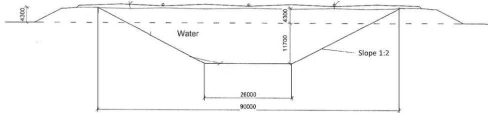
**Figure 3.3. Main geometry parameters of the PTES in Dronninglund.**
