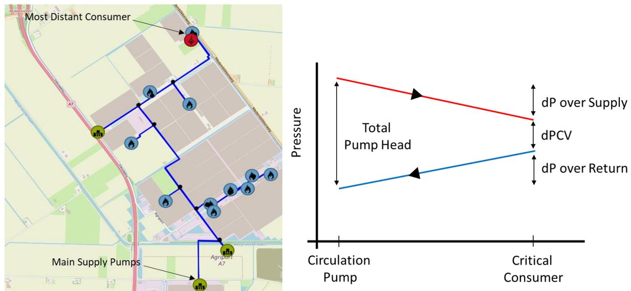
**Figure 2.3. The flow system in ECW Middenmeer and the evolution of the pressure drop over the pipelines.**
