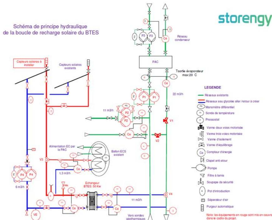
Figure 4.1 : Hydraulic diagram of existing facility (top) and changes that will be done (BTESmart project).
