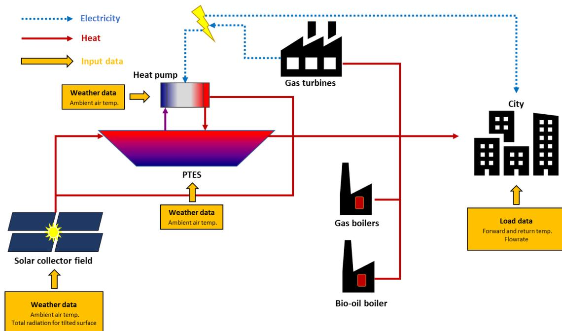
**Figure 3.8. Schematic showing the main elements of the system model for Dronninglund and which elements they can deliver heat to, together with their necessary input data.**
