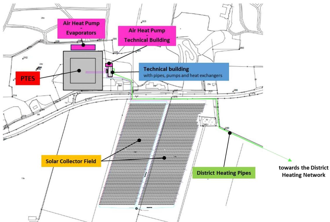
Figure 3.1. Schematic aerial view of the solar and heat pump part of the heating system in Dronninglund.
