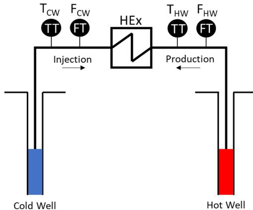
**Figure 2.2. Illustration of measurement locations.**
