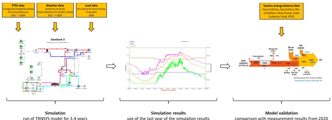
**Figure 3.9. Graphical representation of the model validation procedure (pictures extracted from Gauthier (2021)).**
