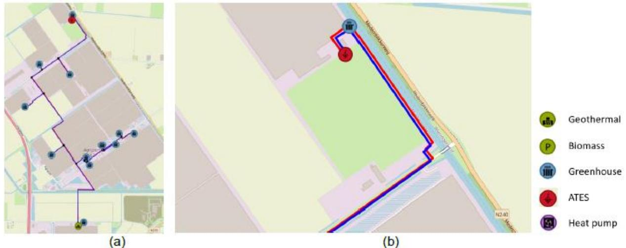
Figure 2.1 a) Schematic overview of the heat network, with the locations of the geothermal sites, the biomass plant, the HT-ATES wells and the heat pump; b) coupling of HT-ATES to the greenhouses.
