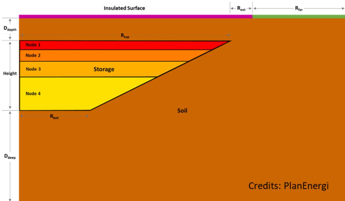
**Figure 3.4. Main parameters used by Type 1300 & 1301, example of implementation with 4 water nodes for the water domain discretization.**
